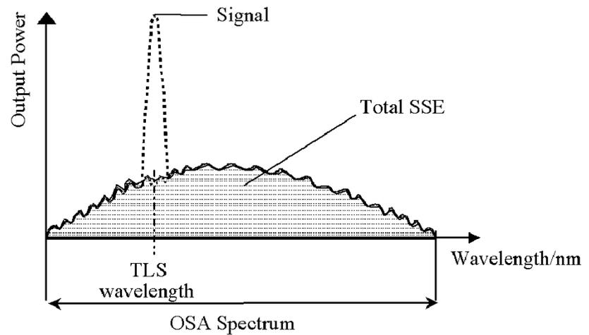
Figure 38 Total SSE Measurement.
