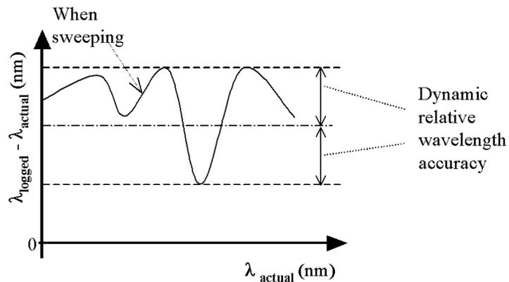
Figure 14 Relative wavelength accuracy (continuous sweep mode).
