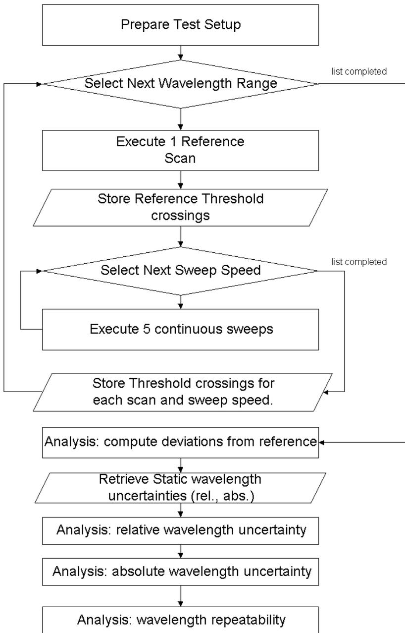
Figure 41 Test Flow - Dynamic Wavelength Accuracy Measurements
