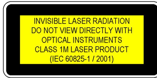
A sheet of laser safety labels is included with the laser module as required. In order to meet the requirements of IEC 60825-1 we recommend that you stick the laser safety labels, in your language, onto a suitable location on the outside of the instrument where they are clearly visible to anyone using the instrument.
