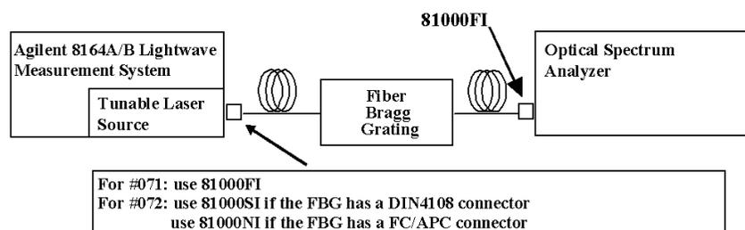
Figure 37 Test Setup for Signal-to-Source Spontaneous Emission Test - Low SSE Output.
