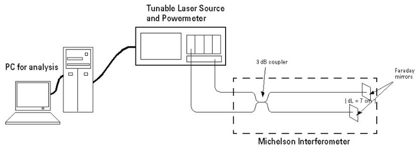
Figure 44 Measurement Setup to Determine the Sweep Speed
