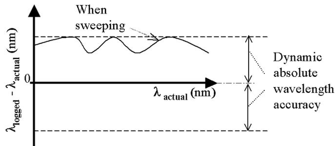
Figure 7 Absolute wavelength accuracy (continuous sweep mode)
