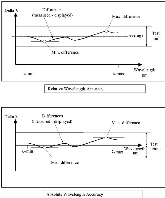
Figure 20 Absolute and Relative Wavelength Accuracy.
