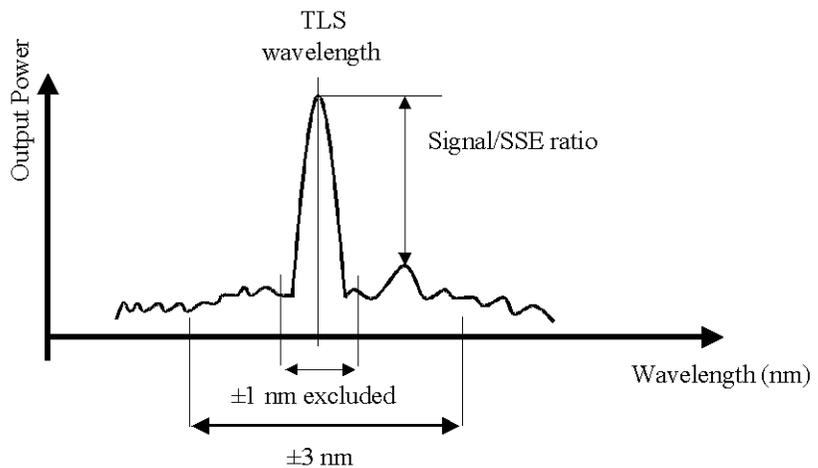
Figure 34 Signal-to-Source Spontaneous Emission Ratio.
