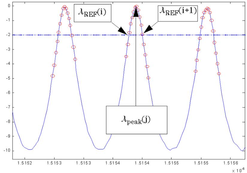
Figure 43 Optimization of reference scans. Sampling points as circled, threshold in dashed line.
