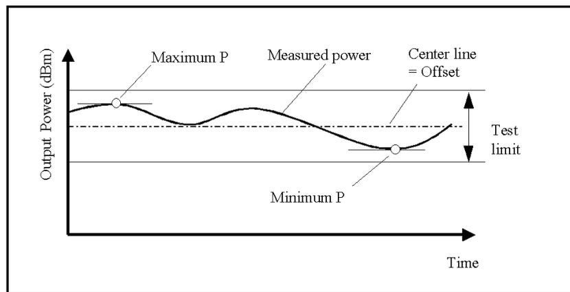
Figure 32 Stability of Power Output versus Time.
