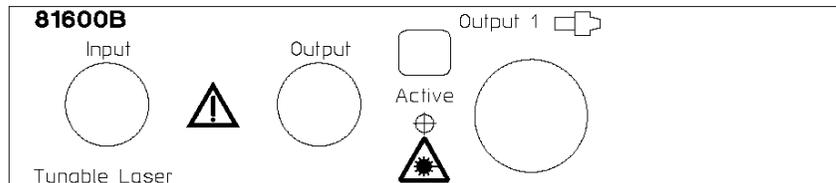
Figure 2 Agilent 81600B Tunable Laser Source Family module
