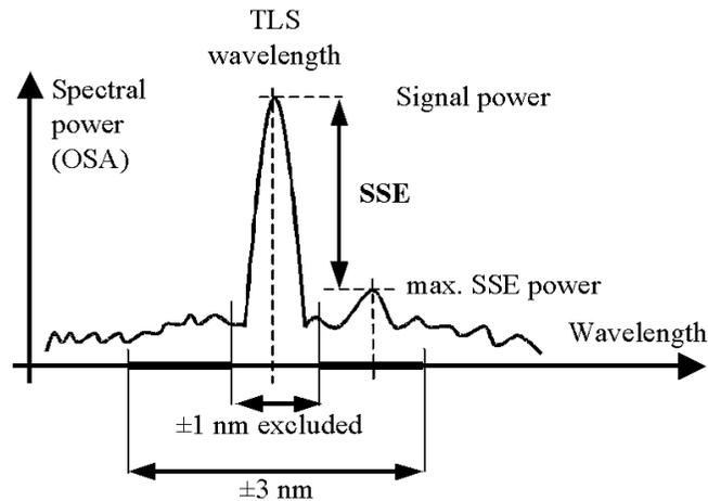
Figure 16 Signal to source spontaneous emission ratio.
