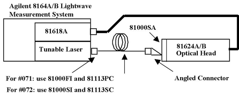
Figure 24 Test Setup for Maximum Output Power Tests
