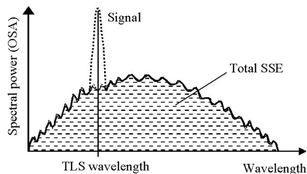
Figure 17 Signal to total source spontaneous emission ratio.
