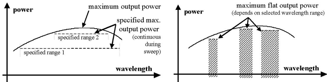
Figure 9 Maximum Output Power vs Wavelength, Maximum Flat Output Power vs Wavelength
