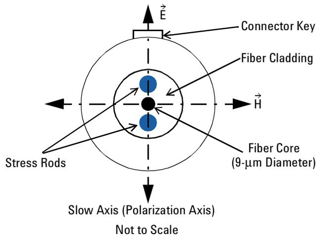
Figure 3 PMF Output Connector
