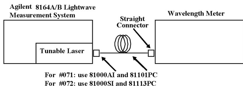
Figure 19 Test Setup for Wavelength Tests
