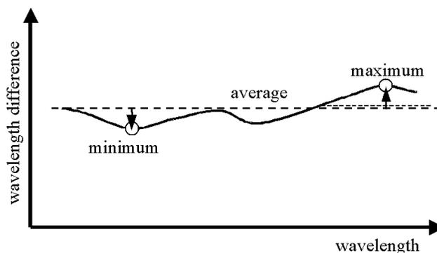
Figure 15 Relative wavelength accuracy.
