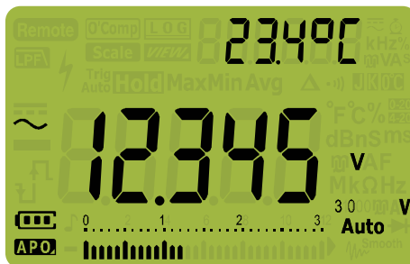
Figure 2-1 AC voltage display
