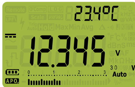
Figure 2-4 DC voltage display
