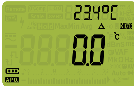
Figure 2-29 Temperature measurement without ambient compensation
