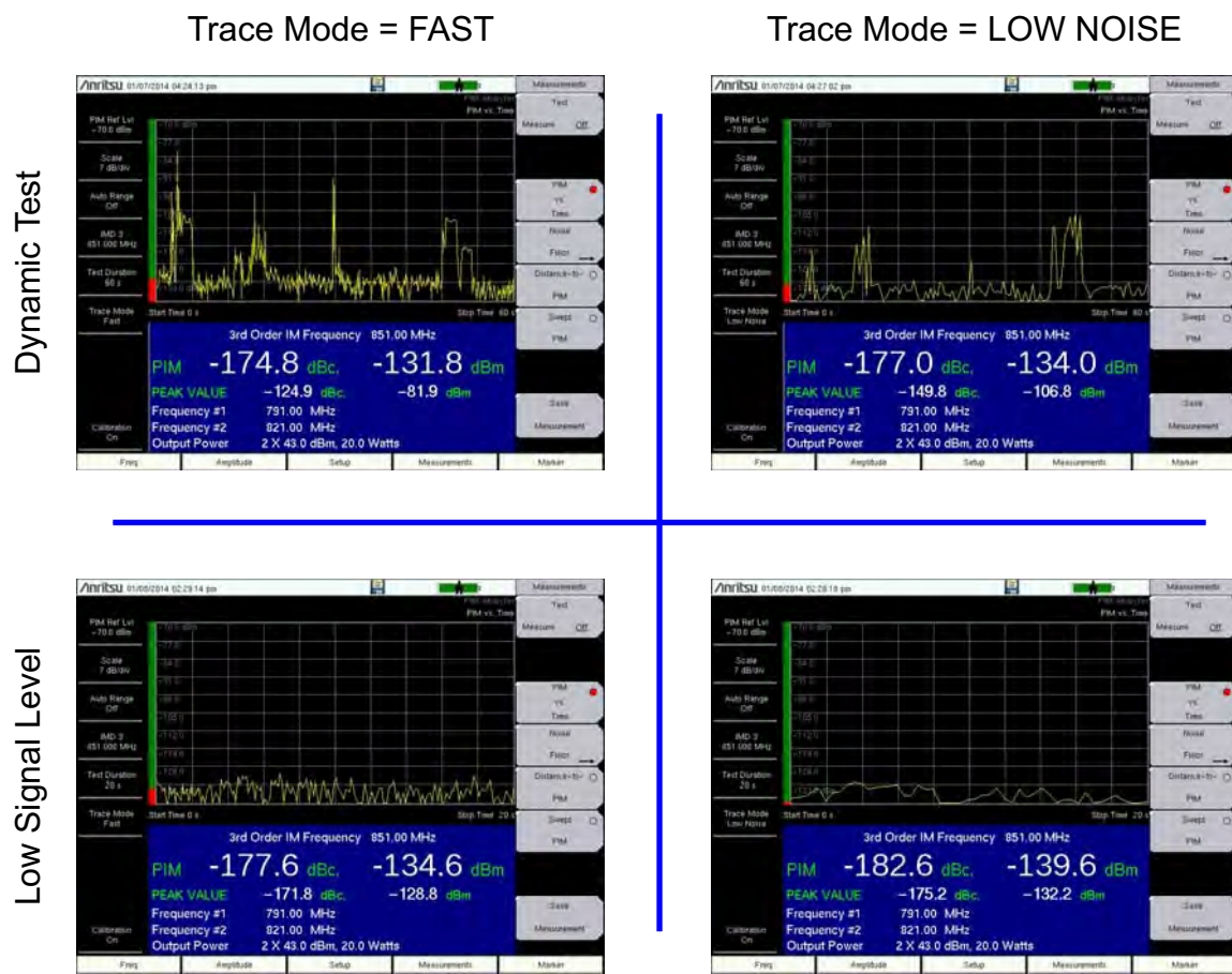
Figure 7-1. Fast and Low Noise Trace Modes
