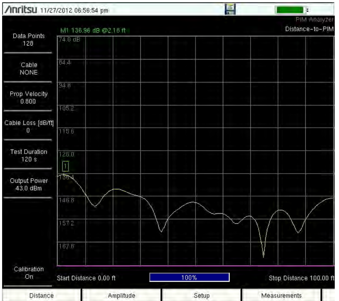
Figure 9-4. Typical DTP Measurement After a Calibration
