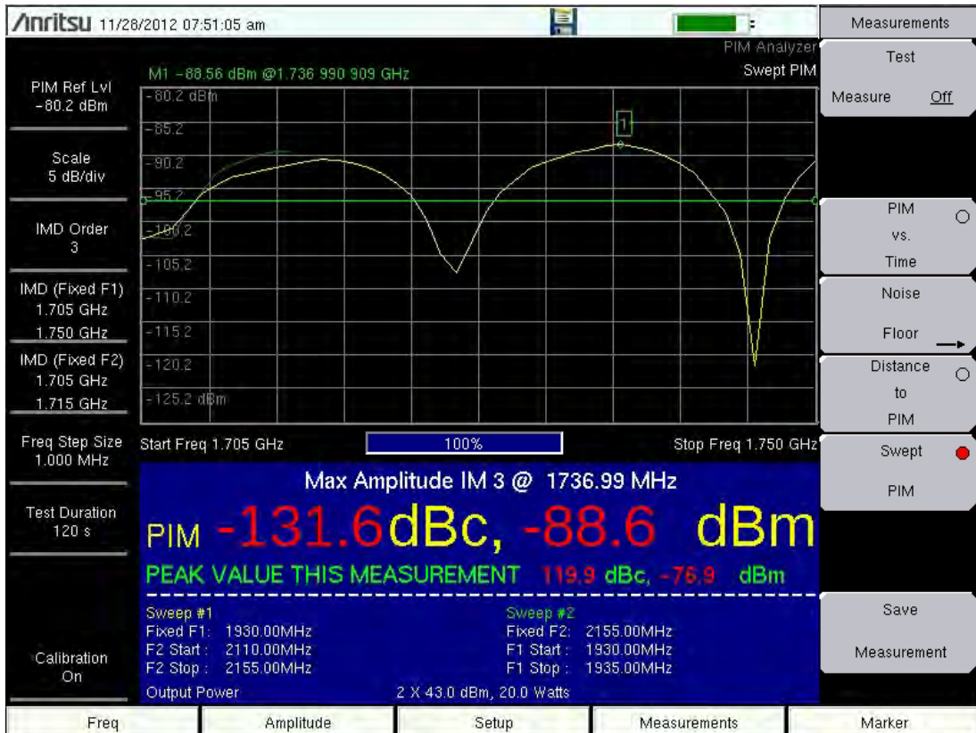
Figure 11-4. Swept PIM IM3 Measurement
