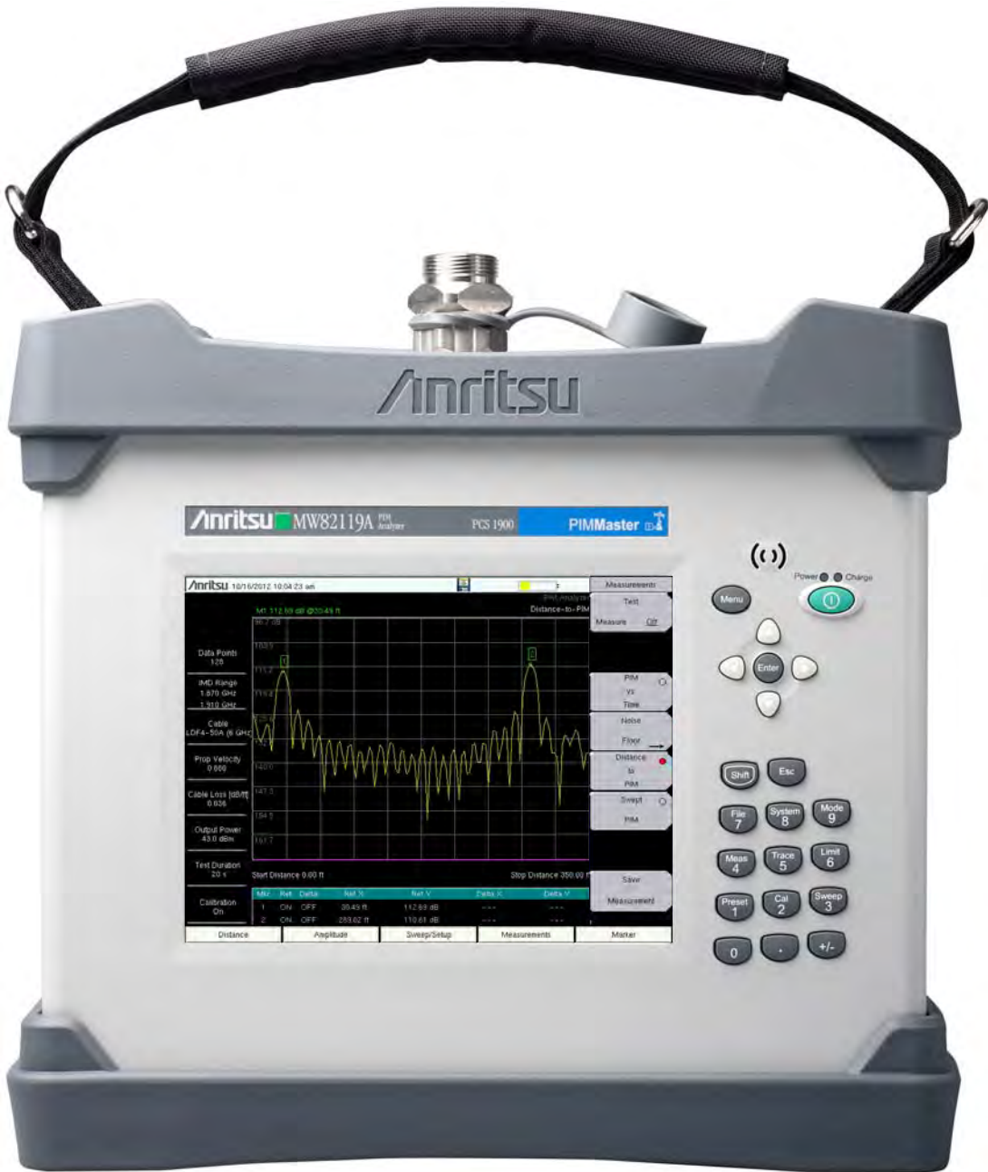
Figure 1-1. MW82119A PIM Master Showing a DTP Measurement
