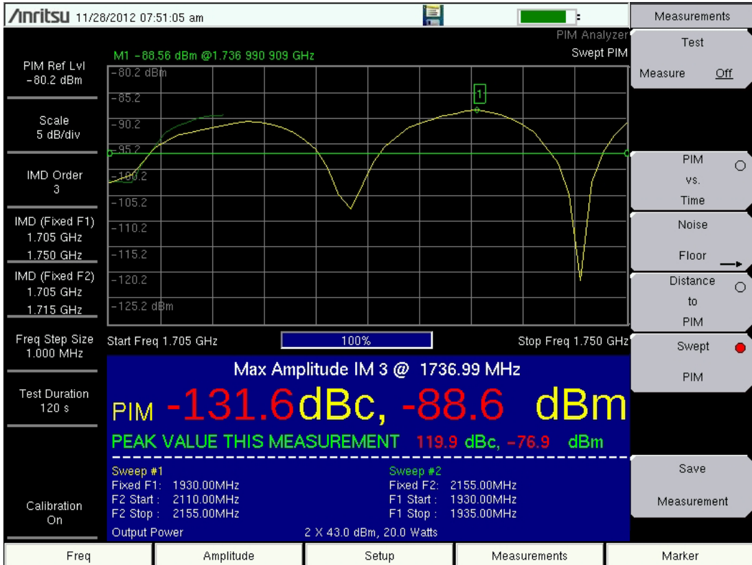
Figure 11-4. Swept PIM IM3 Measurement
