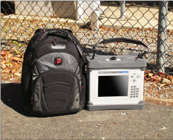
PIM Master MW82119A 40 Watts, Battery-operated
